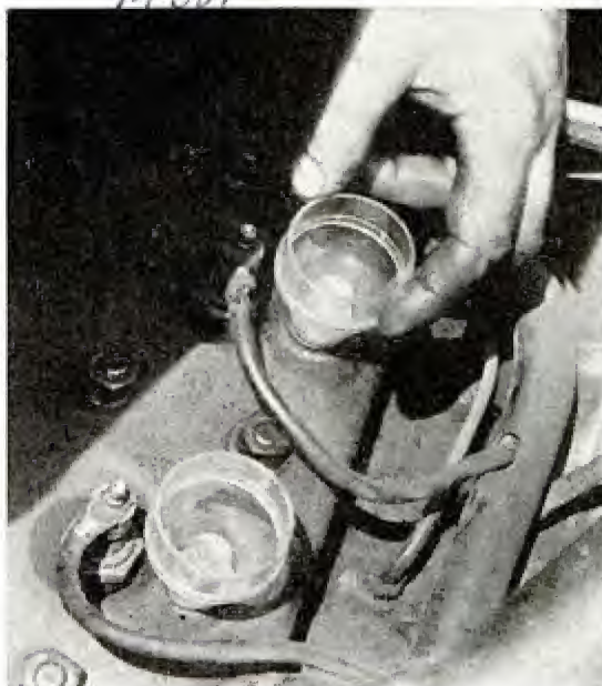
Cup dispenses solvent to free sticking auto stud
